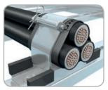
**9** Align the holes of the winding key and retaining bush and put retaining pin through holes until it clips over bush, locking the winding key in place
